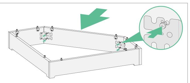
Align the front kickboard piece with the assembly and connect using the provided screws through the bracket slots.
