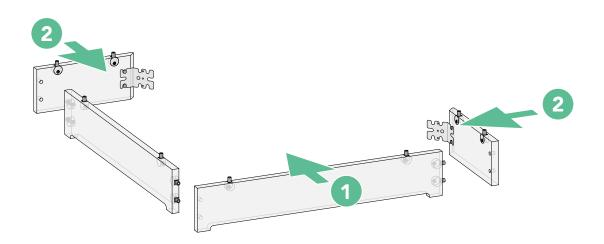
Connect side and back toes of kickboard by aligning cams with their respective sockets and turn phillips head screw in cam clockwise to lock part in place.
