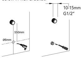
2. Apply thread tape and screw on diverter valve.
