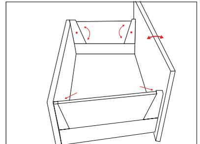
To tilt drawer front, turn adjustment screws on inside of drawer at the front and back, on both sides.
