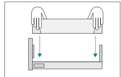
Slide the drawer sides down onto the fixing brackets until the lug secures side in place. Repeat on both sides.
