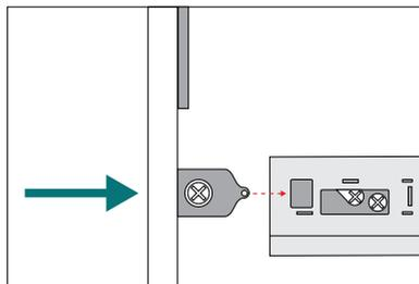
**To replace drawer front:** Align front panel with drawer sides, apply some pressure at the bottom on both sides and push in to secure.
