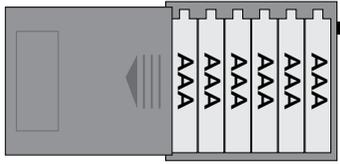
6 x AAA batteries are required for the battery pack. Slide the cover plate off, insert batteries and slide cover plate back on.
