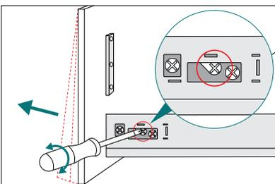
**To remove drawer front:** Turn centre screw and pull drawer front forwards. Repeat on other side.
