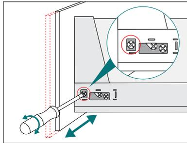
To move drawer front to the right, turn right screw clockwise and left screw anti-clockwise. Turn the opposite way to move to the left.
