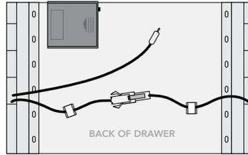
On the back of the drawer attach the supplied battery pack on the top left hand side over the back panel.
