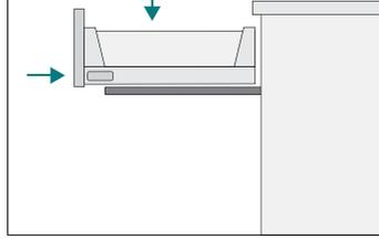
Extend drawer runners out and place drawer on runners and push closed until it is about 2cm out from the vanity. Apply a little extra force on the drawer front (near the bottom of drawer) to push closed
