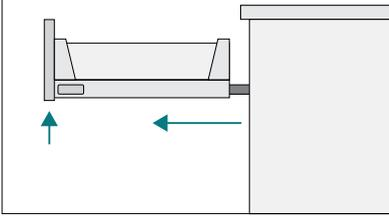
Pull drawer all the way out then lift the front up, a little force is needed to release the drawer from the runner.
