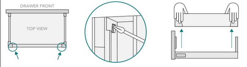
Identify plastic lugs - lugs are at the back of the drawer on each side at the top.
