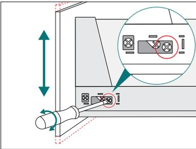
Remove ADP cap to access screws. Turn the back screw to adjust the height of the drawer front. Turn clockwise to go up and anti-clockwise to go down.
