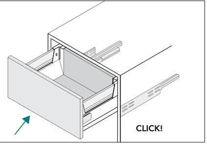
and connect runners in place. The drawer should then be automatically connected to the runner by the two catches. Listen for a click!
