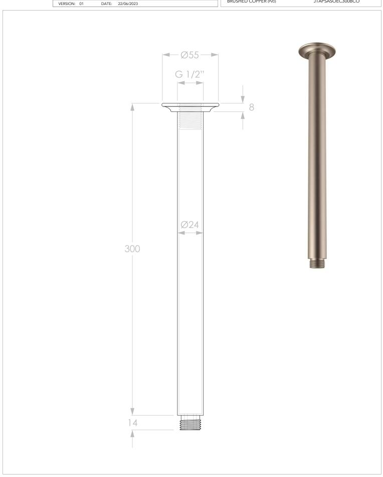
WORKING PRESSURE: 350 – 500KPA (INCLUDING COLD AND HOT WATER PRESSURE)
