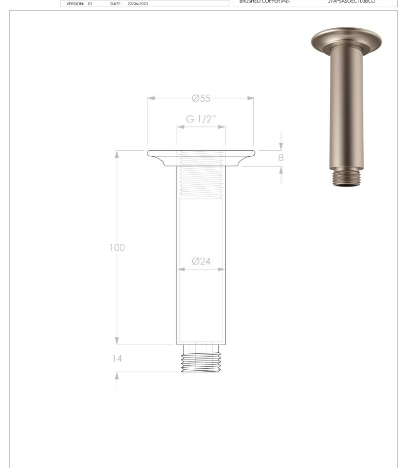
WORKING PRESSURE: 350 – 500KPA (INCLUDING COLD AND HOT WATER PRESSURE)
