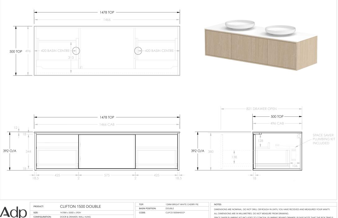
SPACE SAVER PLUMBING KIT INCLUDED TO CONCEAL PLUMBING BEHIND DRAWER. PLEASE NOTE THAT THE BOX TRAP IS NOT COMPATIBLE WITH ALL BASINS. RECOMMEND USING A SHORT TRAP FOR SEMI INSET BASINS.
