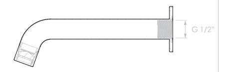
WORKING PRESSURE: 350 – 500KPA (INCLUDING COLD AND HOT WATER PRESSURE)
