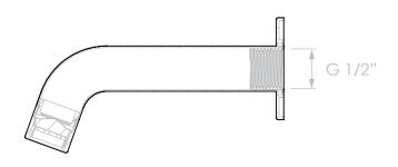
WORKING PRESSURE: 350 – 500KPA (INCLUDING COLD AND HOT WATER PRESSURE)
