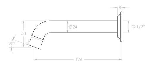
WORKING PRESSURE: 350 – 500KPA (INCLUDING COLD AND HOT WATER PRESSURE)
