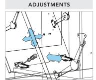
Make door adjustments using the lower hinges.
