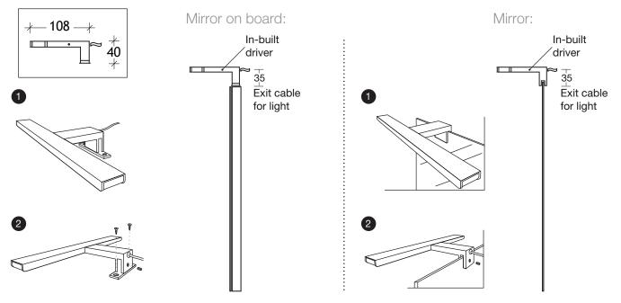
Using standard holder, position light on mirror. Fasten to mirror with screws provided.
