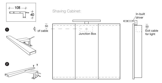
Using standard holder, position light on cabinet as far forward as possible (recommended). Fasten to cabinet with screws provided.
