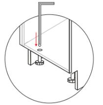
Adjustable metal feet are provided for easily adjusting cabinet levels. Adjustments can be made 30mm up or down.
