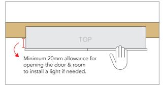
Ensure the cabinet carcass protrudes by a minimum of 20mm from the wall (including tiles) to allow for finger pull on the door.
