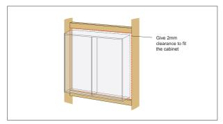
Complete Step 1, cut a hole 4mm bigger than the overall cabinet carcass in the wall. Position and secure cabinet in cut out, go to Step 2.
