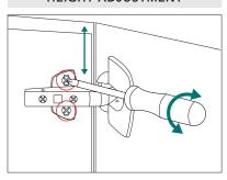
Loosen the top and bottom screw on mount plate, adjust door height by moving door up or down, then retighten screws.
