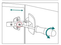
Use front screw to move door to the left or right, or to level each door.
