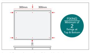
Securely fasten cabinet to the wall through back with appropriate screws/bolts at TOP and BOTTOM of cabinet. Evenly space apart the horizontal fixings at a maximum of 300mm apart.
